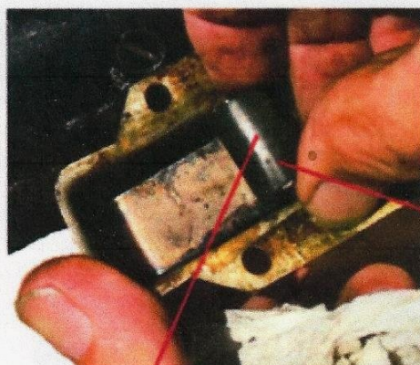
The hose adds more positive spring action to the switch's metal contact strip.
