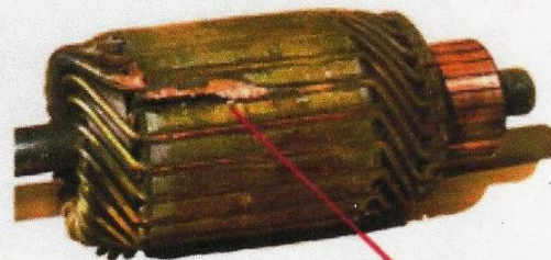
The armature, in this case, was also damaged from the extreme heat that builds up until you can find a way to break the circuit.
