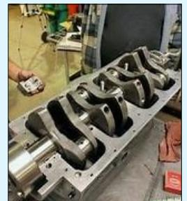
Sep 23, 2021 · Re-Engineering the Model A Engine. Long time MAFCFA member Terry Burtz of Campbell California has long been working on a project to have a **new Model A engine block**, crankshaft and connecting rods manufactured. The engine will be identical to the original Model A engine on the outside but will have 5 main bearings, a balanced crankshaft, and full pressurized oil system
